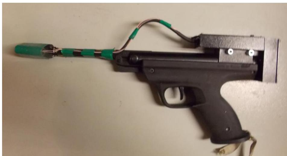
Fig. S6. The Sigma-ART acoustic level meter used to measure the level of drilling fluid in the Vostok borehole.
