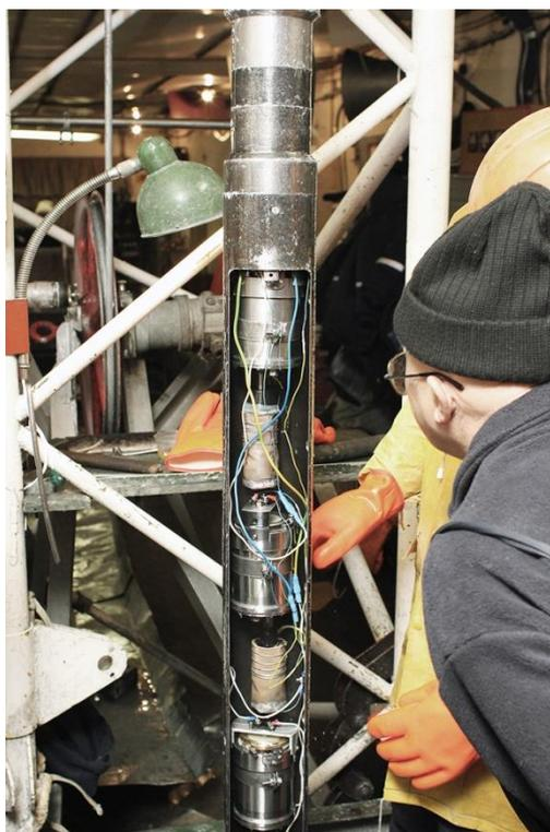
Fig. S1. The three-section downhole drilling fluid sampler.
